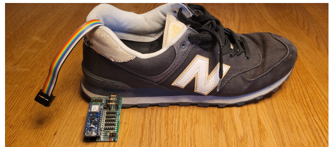
Figure 1: The shoe wearable biometric system, the Arduino board it is attached on the heel of the shoe.
